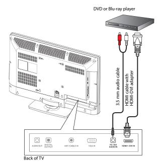
4 Connect an audio cable with a 3.5 mm stereo mini-jack (not included) to the PC/DVI AUDIO IN jack on the back of your TV and to the AUDIO OUT jack on the DVD or Blu-ray player.
